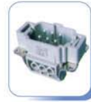
SDC6M 6+1 ♂ Male 500V / 10A Screw Connection
